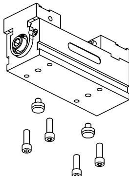
In its basic version, the KSO has 2 x Ø8 H7 positioning holes with which to position it on grid plates with a grid of 50 and in T-slot tables. The KSO is fixed from below using 4 No. M8 cylinder screws.
