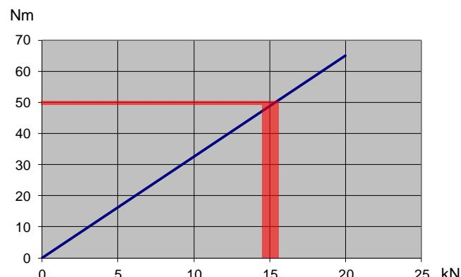
Exposure to loads in excess of the max. pull-in torque results in damage to the spindle.
